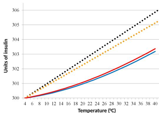
Figure 1: Modeling of heating an empty 3mL cartridge and 3mLs of distilled water or 1% saline from 4 to 40°C. The dotted lines are the empty cartridge volume, with the black dots = linear coefficient of expansion (LCTE) of 180 X 10<sup>-6</sup>, and the orange dots LCTE = 146 X 10<sup>-6</sup>. The solid blue line is 3mLs distilled water and the red solid line is 3mLs 1% saline.
