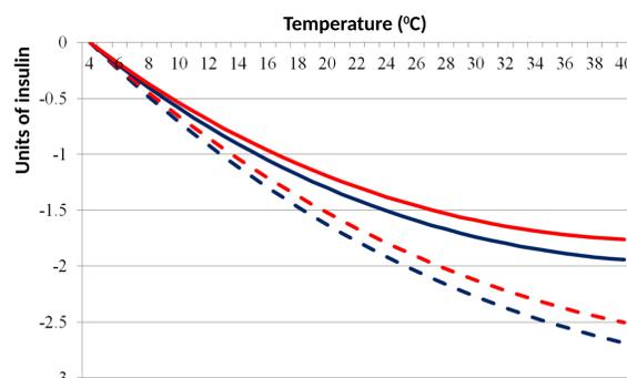
Figure 2: Modeling of heating a 3mL cartridge containing distilled water or 1% saline from 4 to 40°C. Blue lines are distilled water and red lines are 1% saline. The dashed lines LCTE = 180 X 10<sup>-6</sup>, the solid line LCTE = 146 X 10<sup>-6</sup>.
