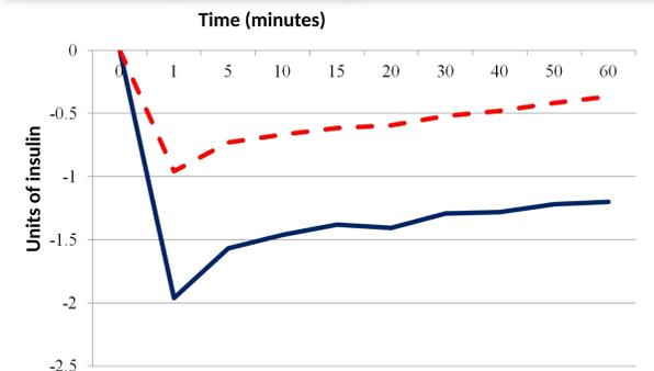
Figure 3: Cartridges for insulin pumps filled with aspart insulin and taken from a refrigerator (4°C) and placed in a water bath (37°C). Solid blue lines are Roche spirit cartridges (3 mL) and dashed red lines are ANIMAS 2020 cartridges (2 mL).
